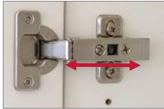
The screw furthest from the door adjusts the hinge back and forth for a flat surface with the other doors.
